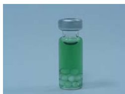
picture 3: SonoCheck before use (negative result)
