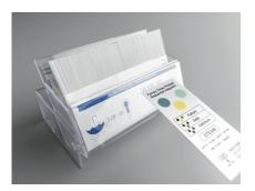
The 3 Phase Integrator (Type 6) comply with **EN ISO 11140-1 Type 1**. 3 Phase Integrators are specially designed to check the time and temperature combination in three different steps & provide a more comprehensive assessment of sterilisation effectiveness (failure, safe & optimum).
