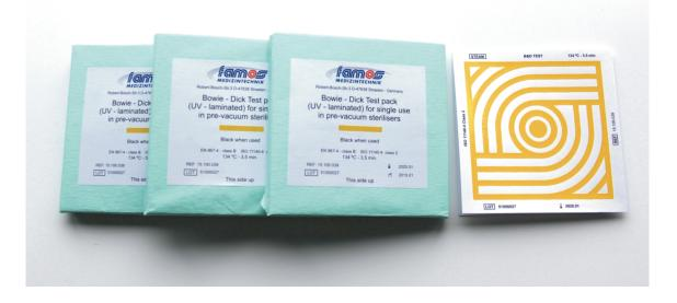
This functionality test for steam sterilisers needs to be done at the beginning of each working day and after a successful pass of the Bowie & Dick Test Pack the steam steriliser can be released for use.
